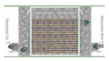
Application : Multi-Door Design is effective when freezing or hardening of Product is done with storage
